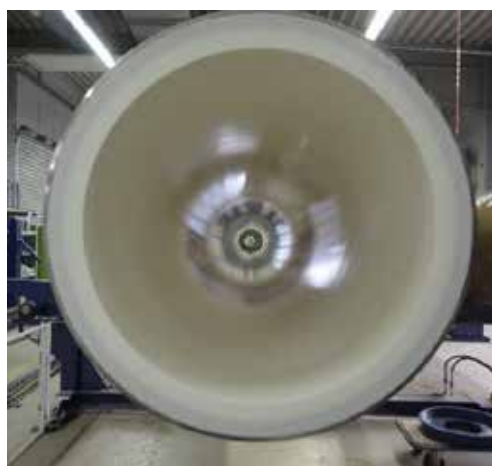
Figure 3: Internally coated pipe for oil sands hydrotransport
