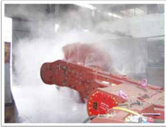
Figure 2 – Air-and-water installation on a shearer
