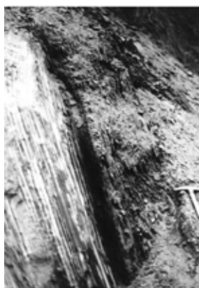
Figure 2 - Unweathered (left) and weathered (right) BIF contact - siliceous itabirite (Ribeiro and Carvalho, 2000)
