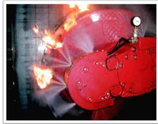
Figure 3 – Extinguishing of flames on a shearer
