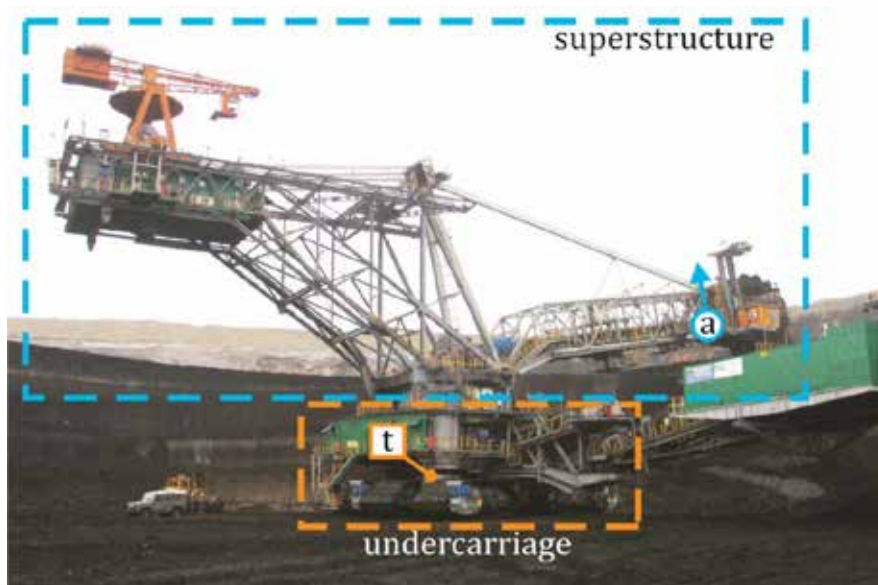
Figure 11 – Superstructure vibration to undercarriage strain relation – testing (a - accelerometer, t - strain gauge)
