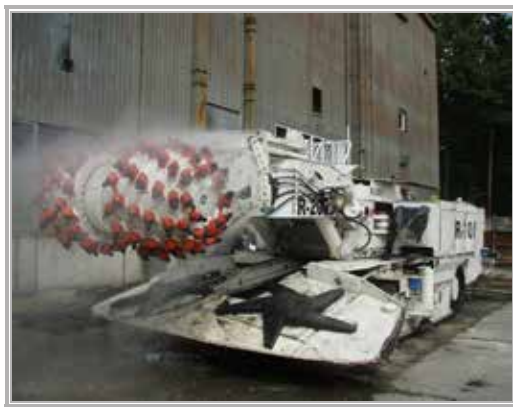
Figure 4 – Air-and-water curtain of roadheader
