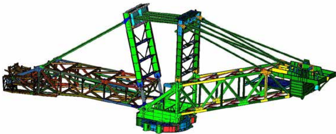
Figure 5 – Finite element model of the bucket wheel excavator
