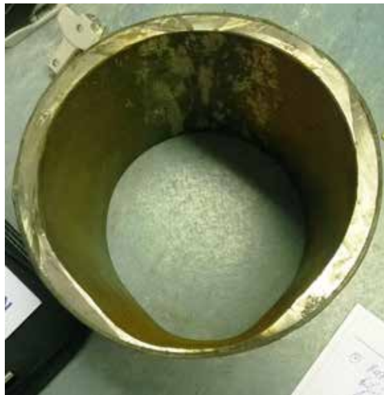
Figure 1: Abrasive wear on steel pipe
