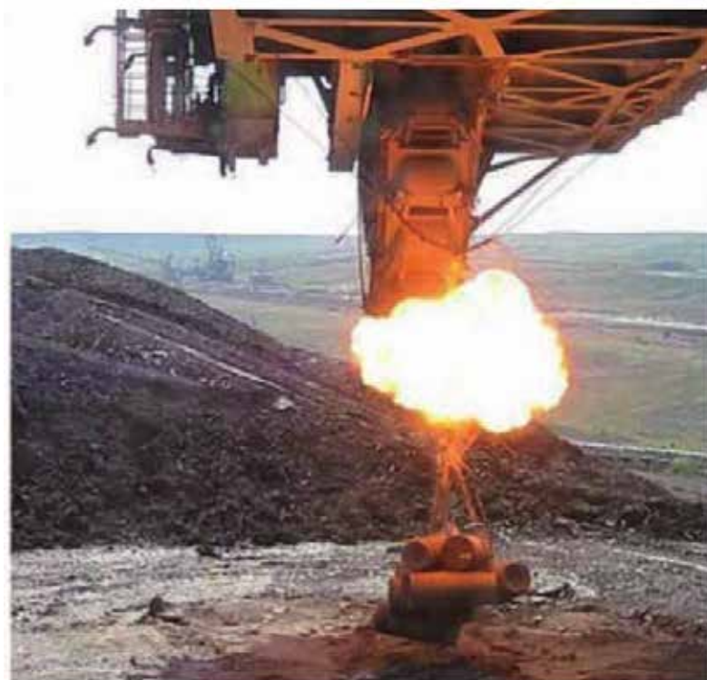
Figure 7 – Mass release with use of explosives (Gottvald, 2010)
