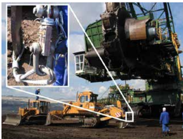
Figure 6 – Mass release with use of the special device (Czmochowski, 2008)
