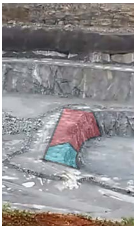
Figure 2 – Bench chosen for study with calcite zone (red) and dolomite zone (blue)
