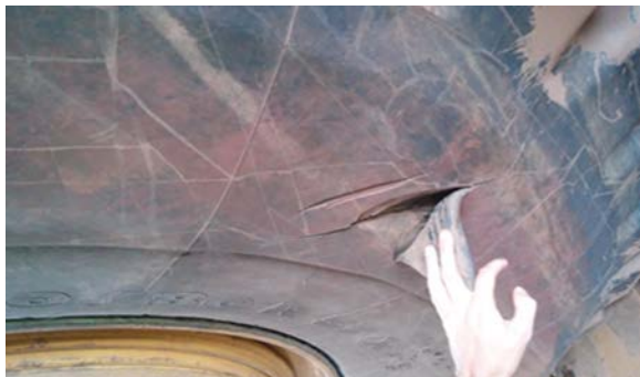
Figure 6 – Truck tire presenting high incidence of side cut
