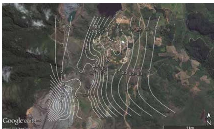
Figure 5 Iso-values of vibrations contour map
