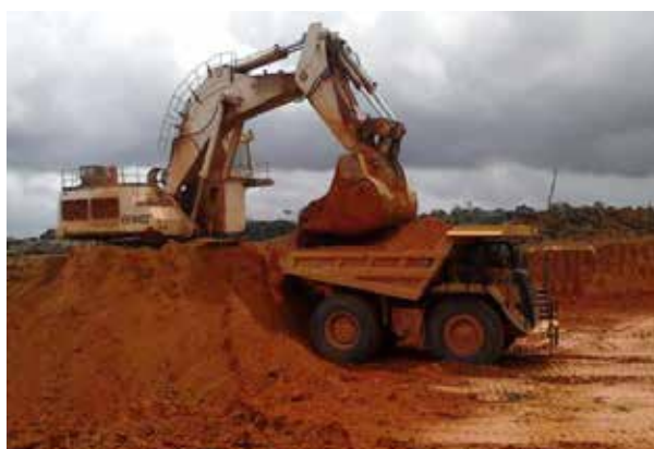
Figure 2 – Stripping using hydraulic excavator + off-road truck
