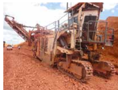
Figure 2 – Surface Miner SM2500 – Wirtgen. Mine of Bauxite - Pará - Brazil. Source: Wirtgen 2014
