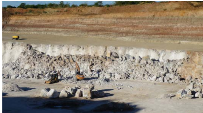
Figure 3 - Mining front of mine Ponta da Serra by Open Pit – Crater Mining method
