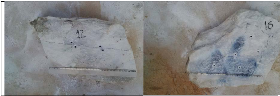
Figure 2. Left: Example of a block with drilling set out to simulate concentrated charges for PF_{th} = 0,3 \text{ kg/m}^3 ; right: Example of a block with drilling set out to simulate distributed charges for P_{.th} = 0,3 \text{ kg/m}^3 .
