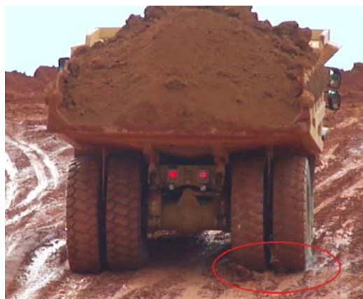
Figure 6 – Absence adherence between the tire and the ground
