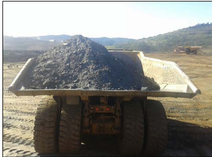
Figure 1: Iron ore decentralized load image at Itabira mines, Brazil.
