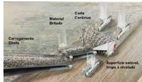
Figure 7 – Cut and load system of surface miner Wirtgen Source: Wirtgen 2014
