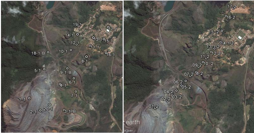
Figure 3 Monitoring points of vibration
