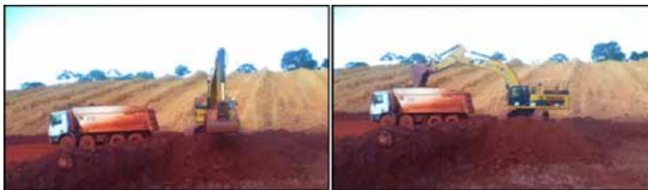
Figure (2) truck-shovel loading with swing angle of 90 degrees.
