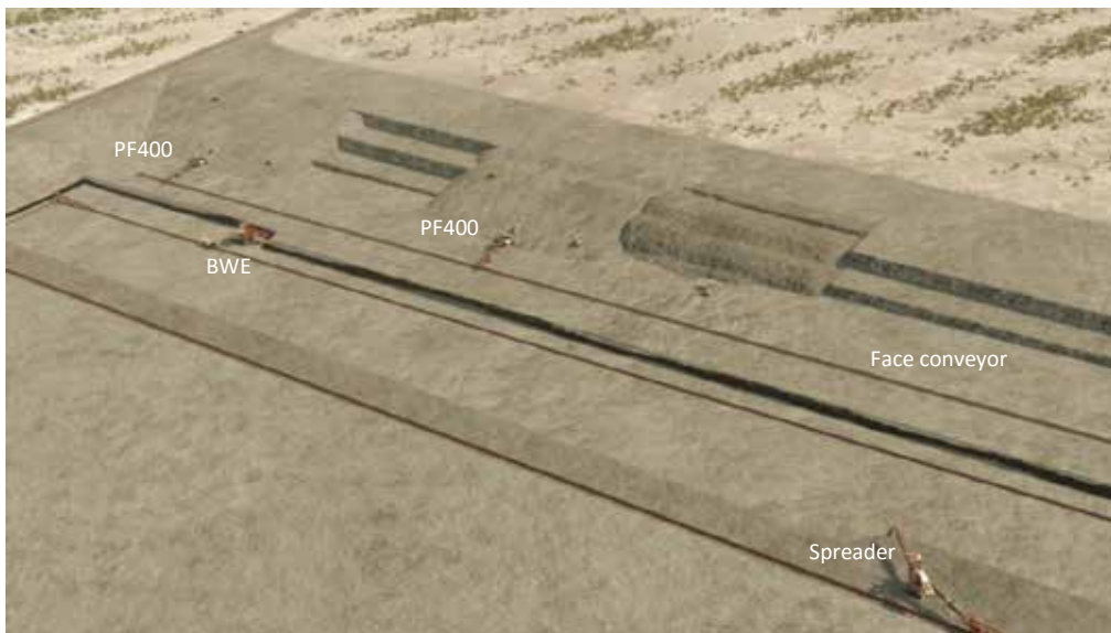
Figure 1 – Example of a mine layout for dozer pushing, using two mobile PF400 crushers, an around-the-pit conveying system, and a spreader for back filling
