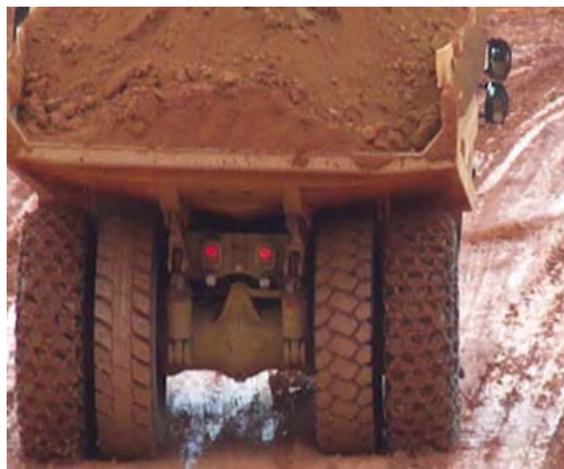
Figure 6 – Tire shielded - greater adherence to contact area
