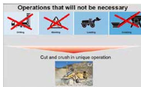
Figure 10: Operations eliminated – Wirtgen Miners Figure 11: Operations eliminated – Vermeer Miners. Source: Adapted from Wirtgen (2010) Source: Adapted from Wirtgen (2010)
