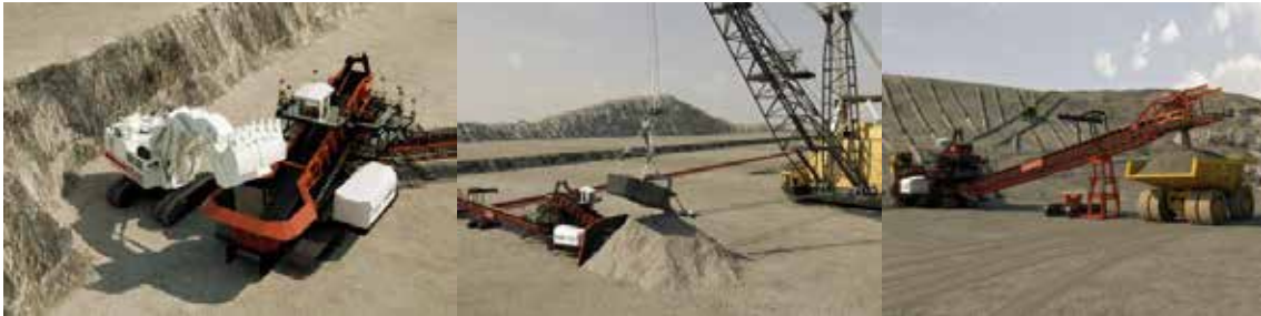
Figure 6 – Alternative usages of the crushing station. Left: Direct shovel feed. Middle: Dragline feed. Right: Discharge to trucks
