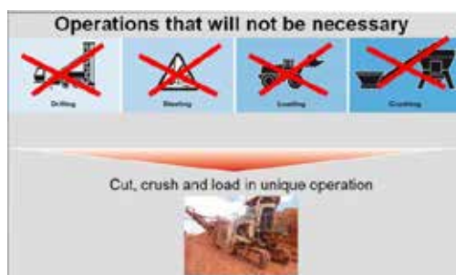
Figure 10: Operations eliminated – Wirtgen Miners Figure 11: Operations eliminated – Vermeer Miners. Source: Adapted from Wirtgen (2010) Source: Adapted from Wirtgen (2010)
