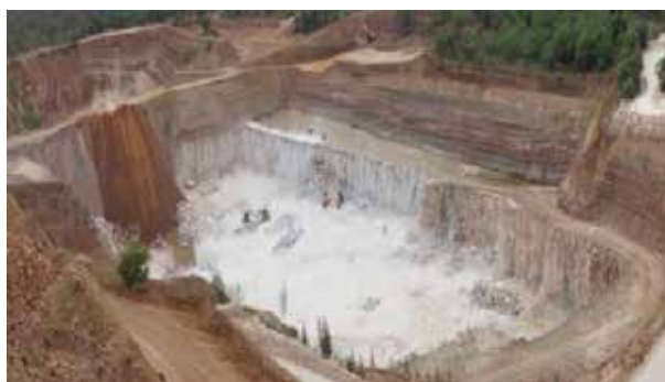
Figure 6 - Deposition of overburden in the pit – Terrace Mining
