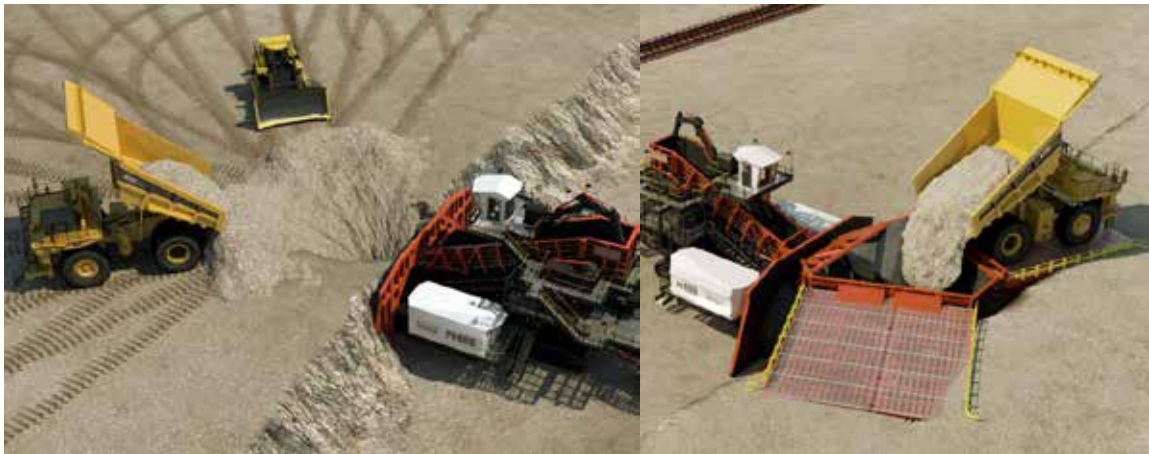
Figure 5 – Truck feed when using the station as a relocatable crusher. Left: Final dozer push. Right: Freestanding hopper
