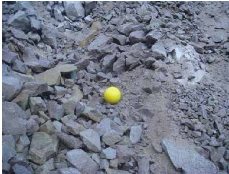
Figure 3: Muckpile image sampling.
