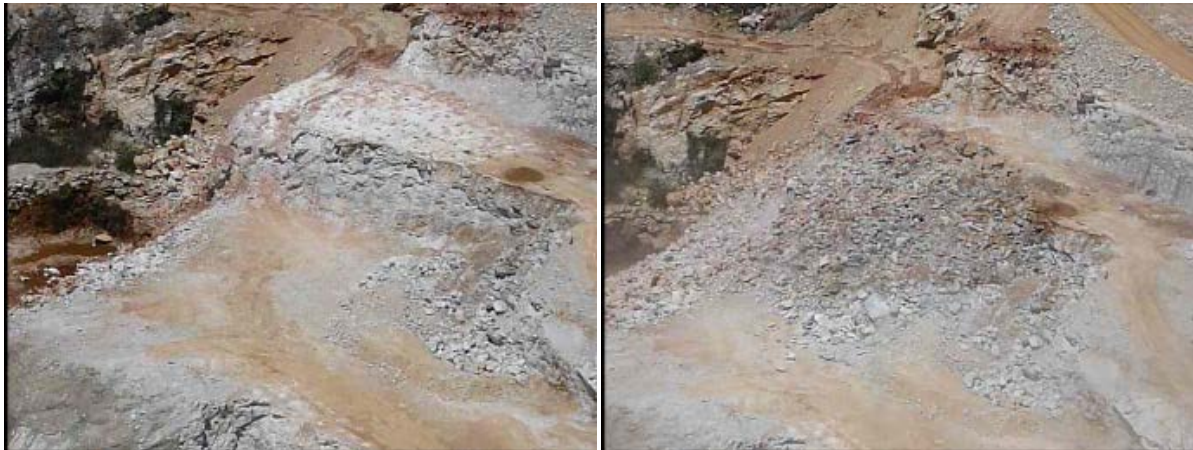
Figure 5. General view of the bench before (left) and after (right) the blast. The free surface, being left by the previous blast, dimensioned according to the proposed method, is smooth and slightly damaged. The muck-pile generated by the blast has a suitable geometry.
