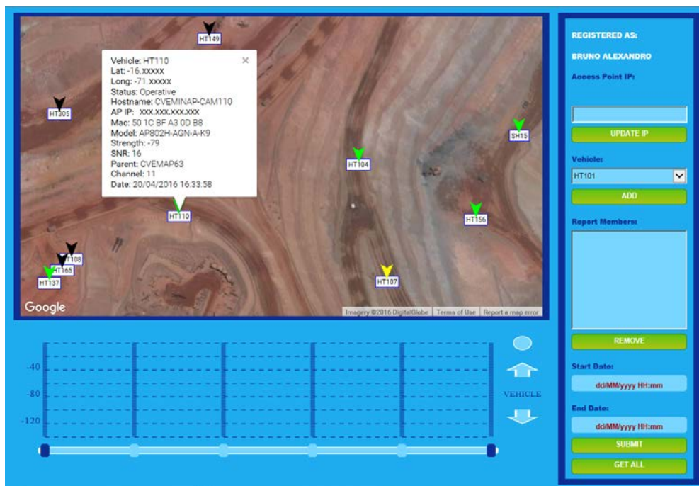
Figure 4 – System main functionality let users check the last reported signal coverage data
