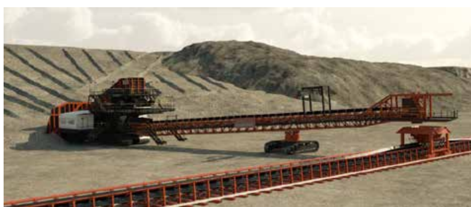
Figure 4 – Crusher and link bridge prior to relocating to a new fan along the face
