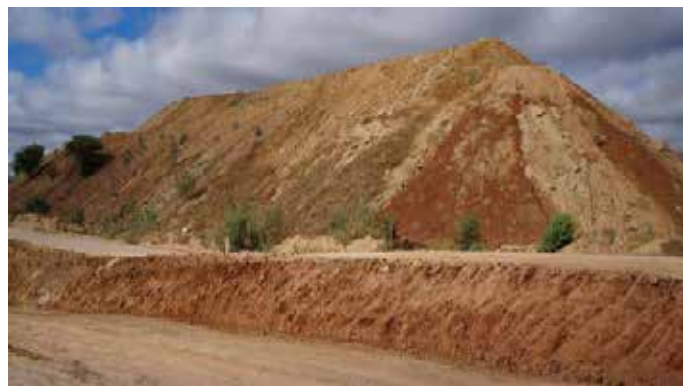
Figure 4 - Overburden bulk resulting of Open Pit – Crater Mining method
