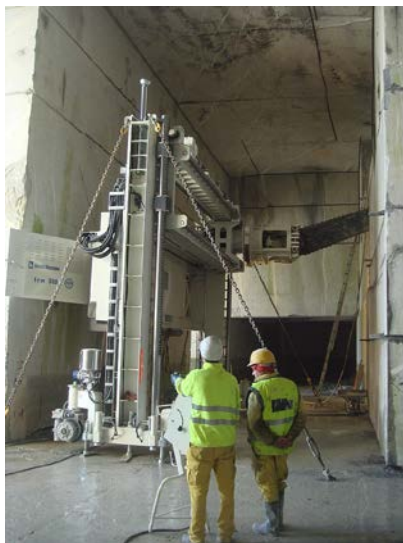
Figure 9 – Benetti chain cutter TCM 988 940
