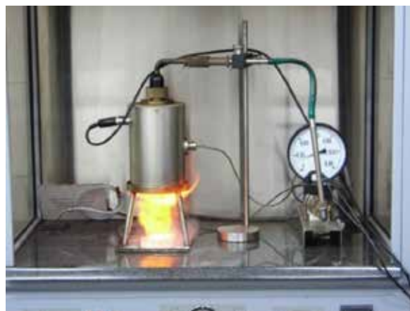
Photo 2. The equipment for the assessment of minimum ignition temperature of a dust cloud
