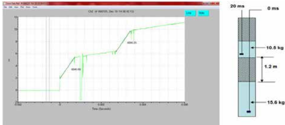
Figure 9. In-the-hole VOD trace of super power 80 cartridge emulsion explosive.
