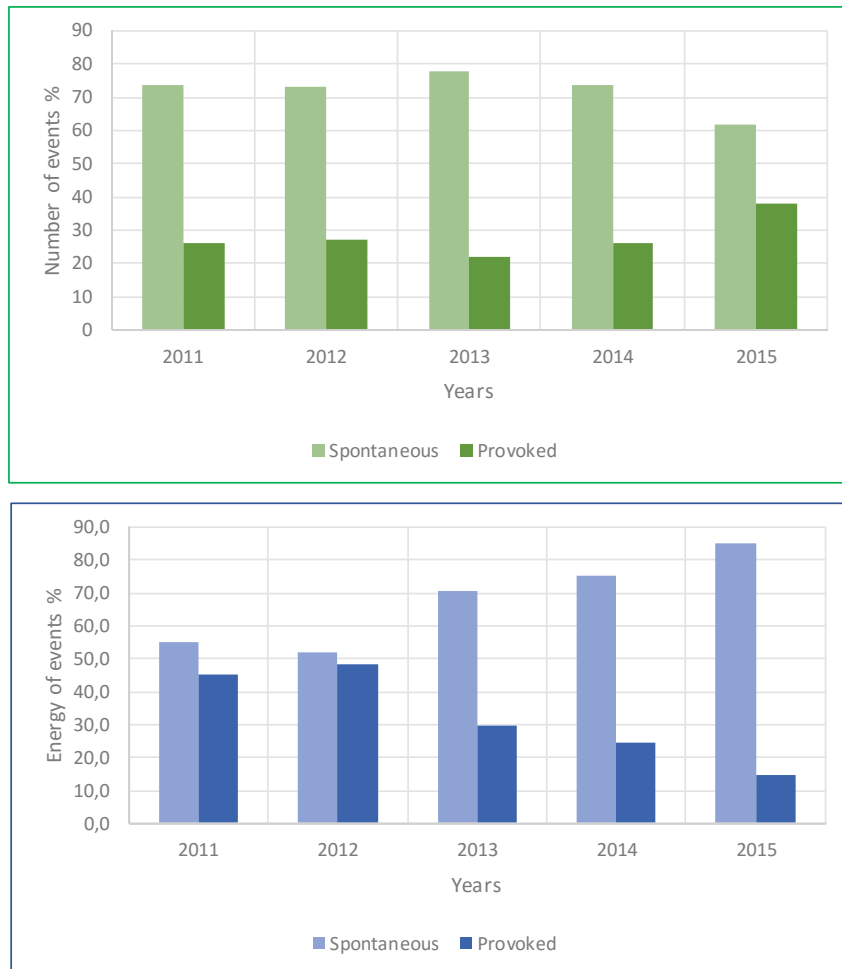
Figure 3 – Effectiveness of the seismic events provoking from point of view of the number of events (top) and their energy emission (bottom) in "Rudna" mine in the years 2011-2015
