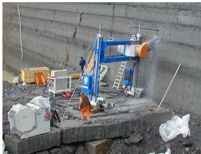
Figure 10 – Benetti diamond belt cutter TCM
