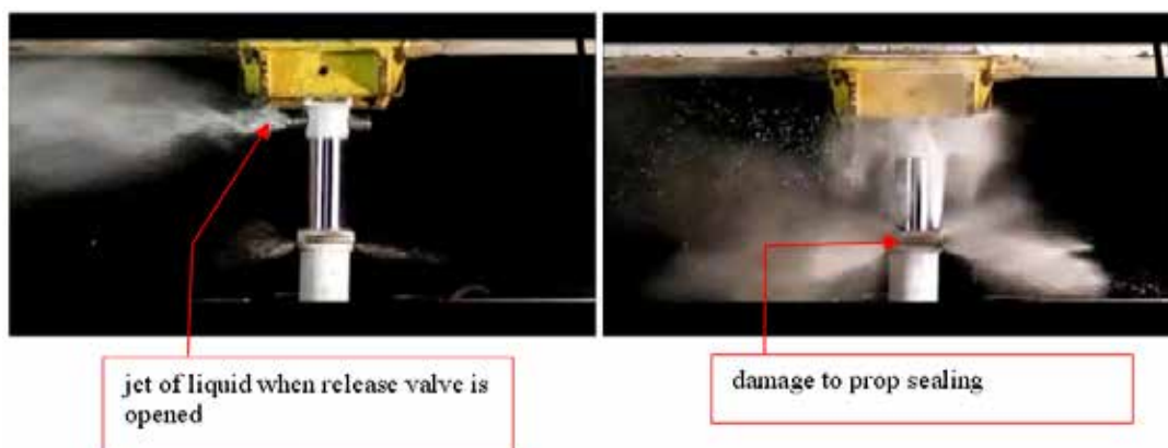
Fig. 6. Destruction of an SHC prop with a working release valve and destruction of sealing in the area above the piston of the prop due to the inadequate performance of the valve (Pytlik 2015b)
