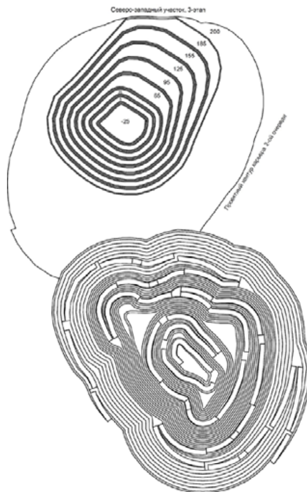
Figure 4 - Alternate mining of Lomonosov mine areas with formation of internal culm dump on mined space of Central region (below North-Eastern region)
