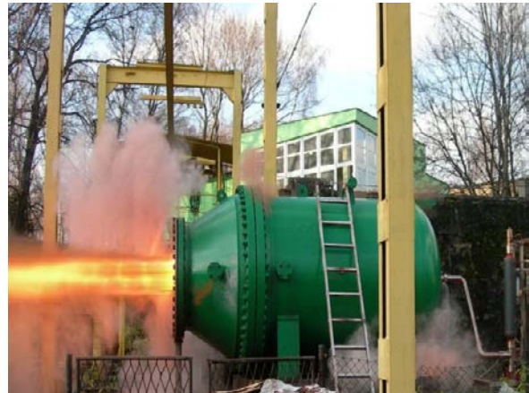
Photo 4. Dust explosion in 5 m 3 vessel used to test explosive properties of dusts, gases and vapors
