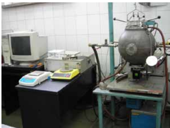
Photo 1. Standard 20-l sphere – the equipment for the assessment dust explosion properties
