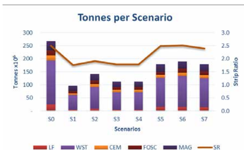
Figure 4 - Total tonnes per scenario and the respective proportion of tonnes of LF (landfill), WST (waste), CEM (cement), FOSC (phoscalcium), MAG (magnesia), SR (strip ratio)
