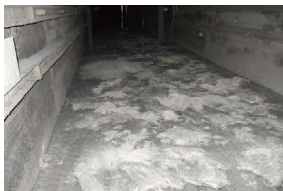
Photo 15. Stone dust barrier with bags placed in an experimental heading at 400 m. after explosion
