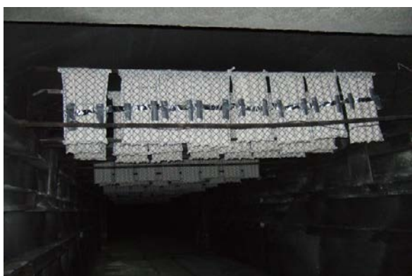
Photo 14. Stone dust barrier with bags placed in an experimental heading at 400 m. before explosion
