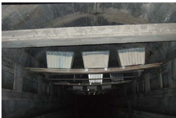
Photo 12. Stone dust barrier with tanks placed in an experimental heading at 400 m. before explosion
