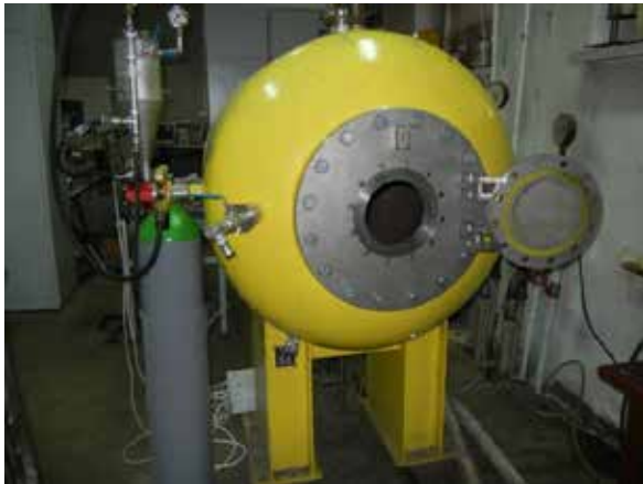
Photo 3. Standard 1 m 3 vessel – the equipment for the assessment of explosion parameters of dusts
