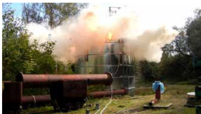
Photo 6. Dust explosion in the grain silo
