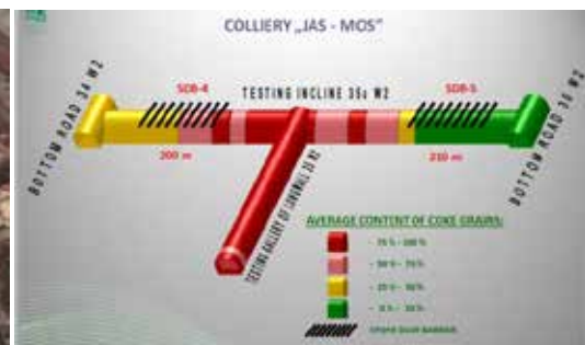
Fig. 1. Jas-Mos colliery – the range of explosion. (SDB- stone dust barrier)
